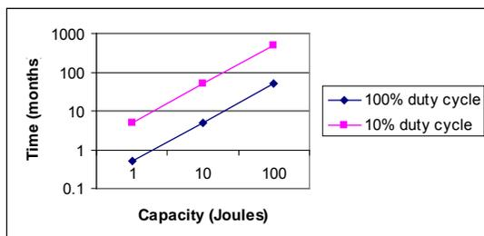
**Figure 1: Maximum time between recharge for 1microwatt of continuous power consumption.**
