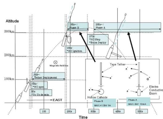
**Fig.1 Experimental Sequence of the S520-25**
