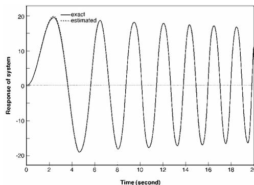
Figure 3. The exact and estimated responses from the first-order discrete time system for a particular first-order dynamic system with a first-order dynamic sinusoidal input.
