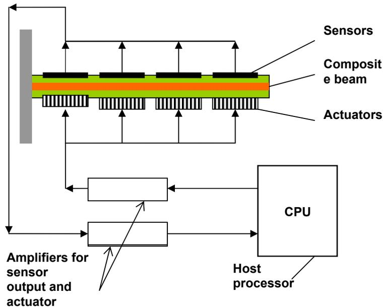
Figure 2. Incorporation of sensor, processor and actuator functions in an intelligent composite beam.
