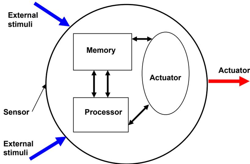
Figure 1. Concept of an "intelligent" material.
