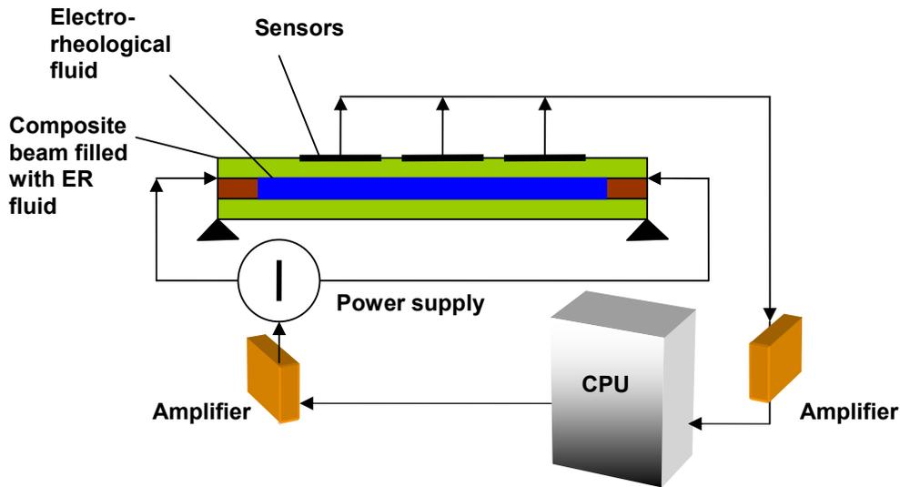
Figure 4. Electrorheological fluid as an actuator in a smart beam.
